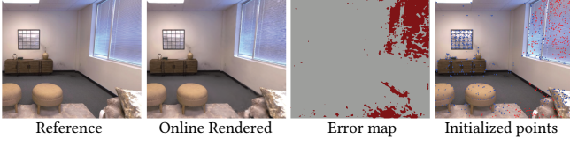
Fig. 3. A visualization of pixels used for initialization. In the error map, red regions indicate high-error areas. In the right-most image, red points represent pixels used for error compensation, while blue points correspond to pixels in geometry- or texture-complex regions.
